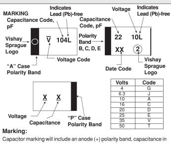
Capacitor marking will include an anode (+) polarity band, capacitance in microfarads and the voltage rating of + 85  $^{\circ}$ C. 'A' Case capacitors use a letter code for the voltage and EIA capacitance code.
