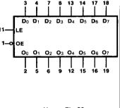
V<sub>CC</sub> = Pin 20 GND = Pin 10
