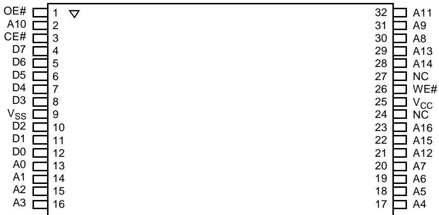
32-Pin TSOP—Reverse Pinout
