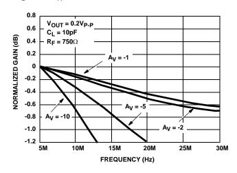
FIGURE 50. INVERTING GAIN FLATNESS vs FREQUENCY
