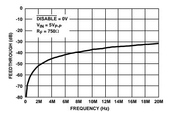
FIGURE 17. DISABLE MODE FEEDTHROUGH vs FREQUENCY
