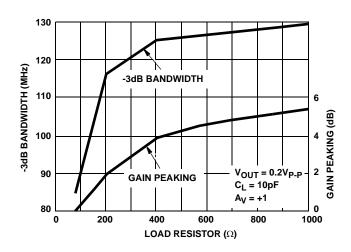
FIGURE 44. BANDWIDTH AND GAIN PEAKING vs LOAD RESISTANCE
