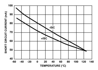
FIGURE 31. SHORT CIRCUIT CURRENT LIMIT vs TEMPERATURE
