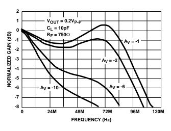
FIGURE 21. INVERTING FREQUENCY RESPONSE
