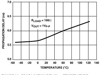
FIGURE 32. PROPAGATION DELAY vs TEMPERATURE (AVERAGE OF 18 UNITS FROM 3 LOTS)
