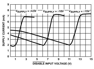
FIGURE 16. SUPPLY CURRENT vs DISABLE INPUT VOLTAGE
