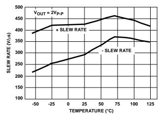
FIGURE 48. SLEW RATE vs TEMPERATURE
