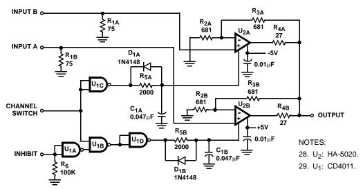
FIGURE 8. LOW IMPEDANCE MULTIPLEXER
