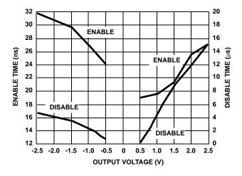
FIGURE 54. ENABLE/DISABLE TIME vs OUTPUT VOLTAGE
