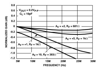
FIGURE 49. NON-INVERTING GAIN FLATNESS vs FREQUENCY
