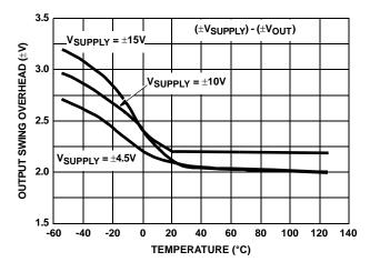
FIGURE 29. OUTPUT SWING OVERHEAD vs TEMPERATURE (AVERAGE OF 30 UNITS FROM 3 LOTS)
