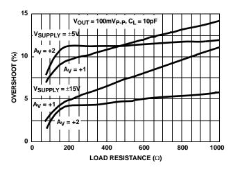
FIGURE 34. SMALL SIGNAL OVERSHOOT vs LOAD RESISTANCE
