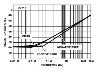
FIGURE 46. REJECTION RATIOS vs FREQUENCY
