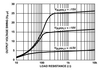
FIGURE 30. OUTPUT VOLTAGE SWING vs LOAD RESISTANCE
