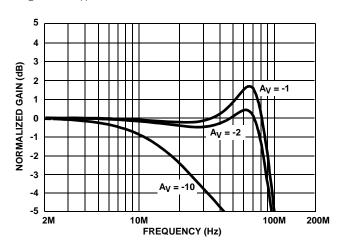
FIGURE 39. NON-INVERTING FREQUENCY RESPONSE
