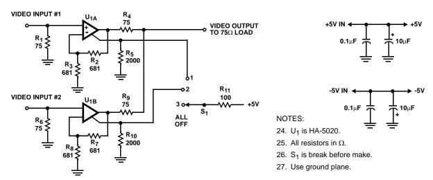
FIGURE 8. TWO CHANNEL HIGH IMPEDANCE MULTIPLEXER
