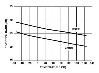
FIGURE 27. REJECTION RATIOS vs TEMPERATURE (AVERAGE OF 30 UNITS FROM 3 LOTS)
