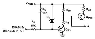
FIGURE 7. SIMPLIFIED SCHEMATIC OF ENABLE/DISABLE **FUNCTION**
