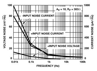
FIGURE 51. INPUT NOISE CHARACTERISTICS
