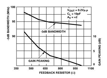
FIGURE 43. BANDWIDTH AND GAIN PEAKING VS FEEDBACK RESISTANCE
