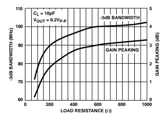
FIGURE 23. BANDWIDTH AND GAIN PEAKING VS LOAD RESISTANCE
