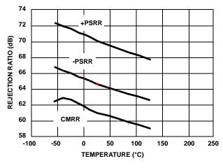
FIGURE 52. REJECTION RATIO vs TEMPERATURE
