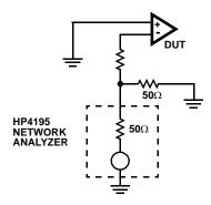
FIGURE 1. TEST CIRCUIT FOR TRANSIMPEDANCE MEASUREMENTS
