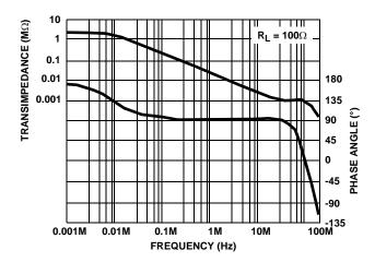
FIGURE 55. DISABLE FEEDTHROUGH vs FREQUENCY
