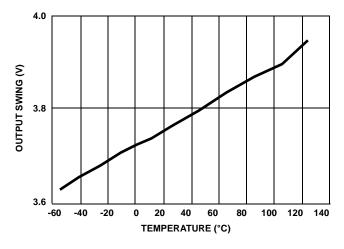
FIGURE 53. OUTPUT SWING vs TEMPERATURE
