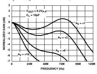
FIGURE 20. NON-INVERTING GAIN vs FREQUENCY
