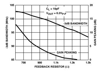
FIGURE 24. BANDWIDTH AND GAIN PEAKING VS FEEDBACK RESISTANCE
