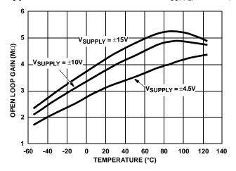
FIGURE 13. TRANSIMPEDANCE vs TEMPERATURE (AVERAGE OF 30 UNITS FROM 3 LOTS)
