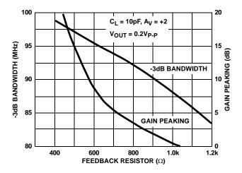
FIGURE 25. BANDWIDTH AND GAIN PEAKING vs FEEDBACK **RESISTANCE**
