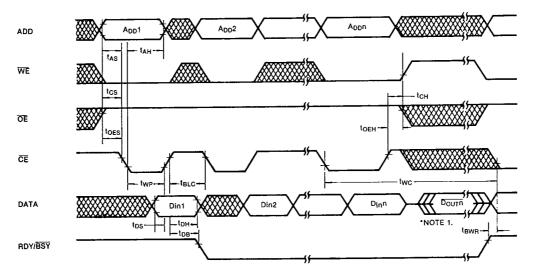
\*Note 1. Tristate for  $I/O_1$ - $I/O_7$ ,  $\overline{D_{out}}^n$  for  $I/O_8$  if the chip is read (see  $\overline{Data}$ -polling)
