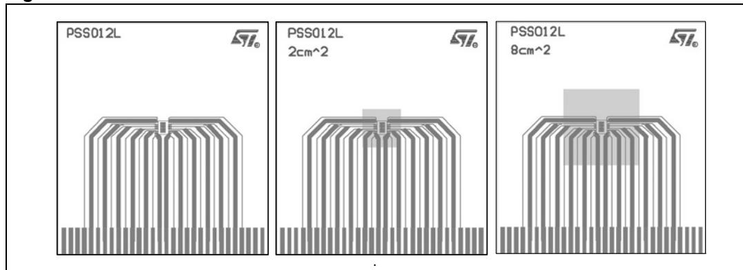
Note: Layout condition of  $R_{th}$  and  $Z_{th}$  measurements (PCB: Double layer, Thermal Vias, FR4 area= 77mm x 86mm, PCB thickness=1.6mm, Cu thickness=70 $\mu$ m (front and back side) Thermal vias separation 1.2 mm, Thermal via diameter 0.3 mm +/- 0.08 mm, Cu thickness on vias 0.025 mm, Footprint dimension 4.1 mm x 6.5 mm).
