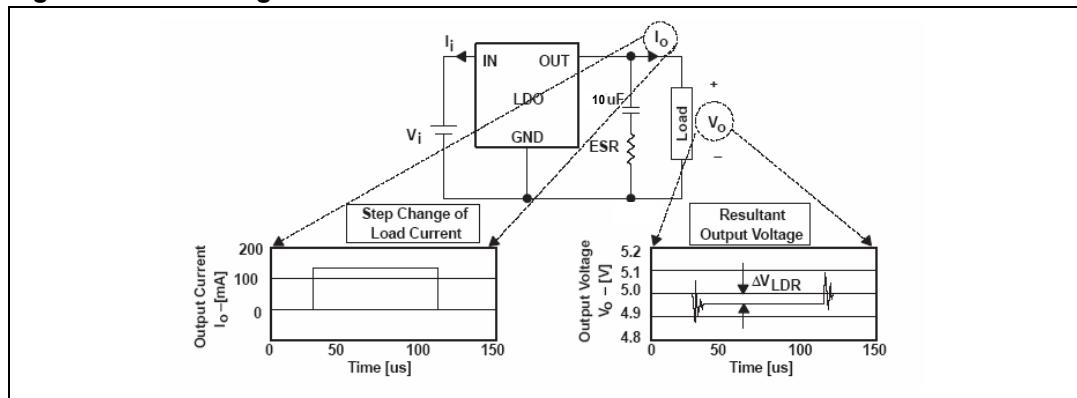
**Figure 25.** Maximum load variation response
