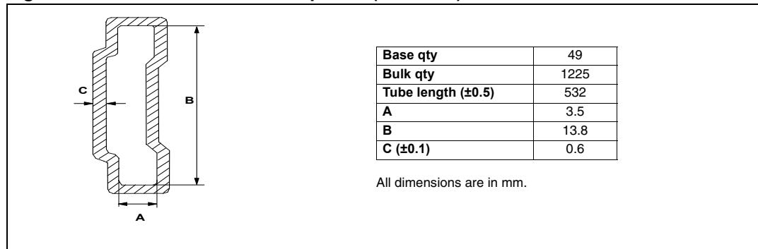
**Figure 43. PowerSSO-24 tape and reel shipment (suffix "TR")**
