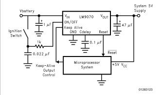
**FIGURE 1. Typical Application Circuit**
