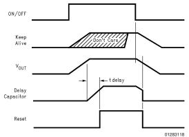
Switch ON with ON/OFF input; Keep output biased with Keep-Alive; Hold ouput ON with ON/OFF; Turn OFF with ON/OFF input. (Temporary Keep-Alive Mode)
