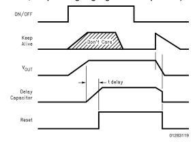
Safety Latch OFF of V<sub>OUT</sub> when in Keep-Alive Mode (ON/OFF going high required to turn Output back ON)
