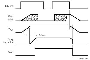
Keep-Alive Mode; Turn ON with ON/OFF control, Keep output biased with Keep-Alive input, Turn OFF with Keep-Alive (Keep-Alive low keeps output ON, Keep-Alive going high turns output OFF)
