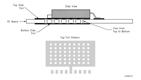
FIGURE 3. Typical TO-263 PC Board Heatsinking
