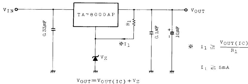
(b) Voltage boost by use of resistor
