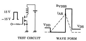
$$\begin{aligned} &RG = 25~\Omega \\ &V_{DD} = 90~V,~L = 43.6~mH \end{aligned} \quad E_{AS} = \frac{1}{2} \cdot L \cdot I^2 \cdot \left( \frac{BVDSS}{BVDSS - VDD} \right) \end{aligned}$$
