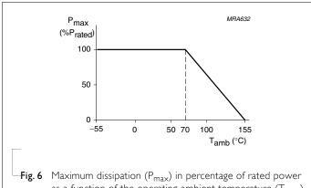
as a function of the operating ambient temperature (T<sub>amb</sub>)
