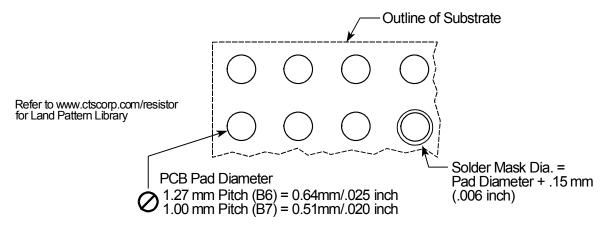
For .006" thick Solder Paste Stencil, Aperture Opening Should be Equal to the PCB Pad Diameter.
